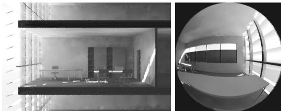
**Figure 6:** Results of luminance images, according to human perception of the eye with solar irradiation. The cross section of the office room and the view from a sitting person at the working place shows how the room looks like when there are louvres in front of the southern facade and a down-to-top roller blind at the windows of the eastern facade. The sun position is scheduled to the 21st March at 10:00 o'clock in Braunschweig Germany (Latitude 52,1° N).
