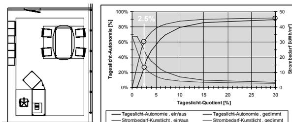
**Figure 7:** Results - daylight factor and daylight autonomy for the office room for the lighting zone of the working area in the lower left of the ground plane
