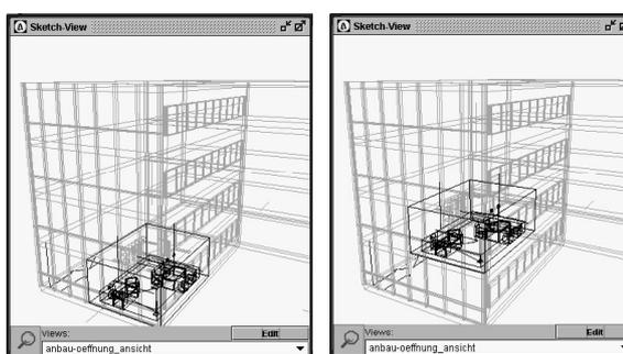
Figure 6: Easy and fast change of geometry - A room with all contained objects can be shifted in a building one floor higher.
