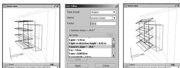
Figure 5: Easy rotation of blinds by changing the louvres-slope angle
